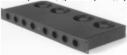
The Cool-cube is a temperature controlled system, and comes with a dual-fan system which senses temperature rise, turning the fan on and off automatically. It can be ordered with 6' of 4" / 6" (i.d./o.d.) tubing. The use of the largest tubing possible in a given installation is highly recommended, as this maximizes air flow while minimizing noise.
